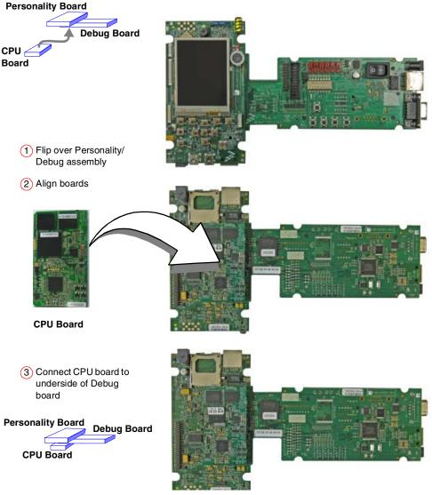
Figure 3.3 Align CPU board and Debug/Personality board
